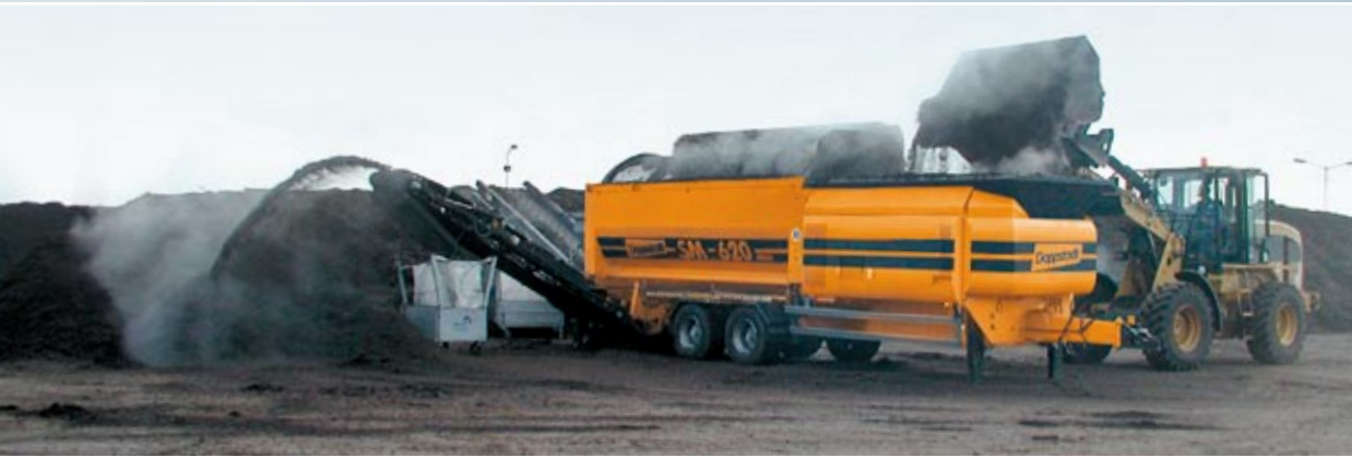
Composting: Separation via rear and side conveyor
