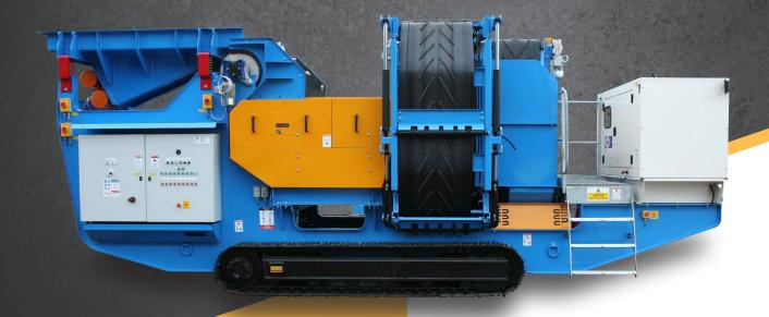
a mobile eddy current separator using a powerful magnetic field to separate ferrous and non-ferrous metals such as aluminium and copper from a variety of materials. Incorporating the
