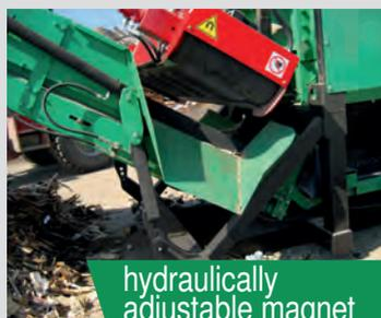
hydraulically adjustable magnet
